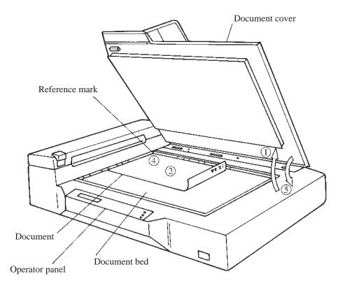
Figure 4.1 Flatbed reading
